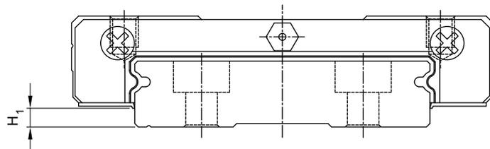
Table 2.52 附防尘片滑块之安装面间隙H<sub>1</sub>
